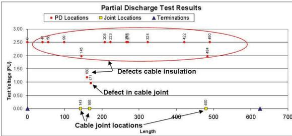
Figure 2 Off-line 50/60Hz PD Diagnostic Test Results
