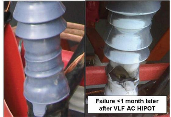
*Figure 1 Cable Termination with Substandard Performance (left)
