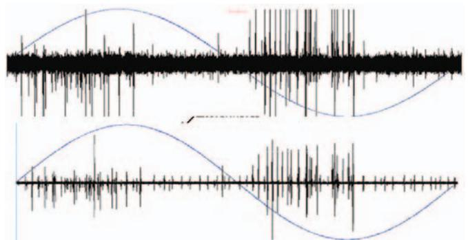
Figure 3. Unprocessed partial discharge (PD) data (above) recorded during one voltage cycle and data after noise mitigation (below).
