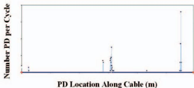
Figure 4. PD histogram showing, at each location, the number of partial discharge (PD) per cycle.
