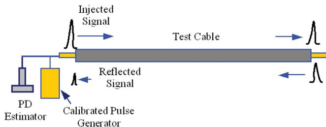
Figure 1. Setup to assess the threshold of sensitivity during a field test.
