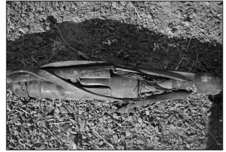
**Figure 2. Partial discharge typically produces defects in the insulation of new cables and between a conductor and a floating metal component, if the electric field is higher than a certain threshold value.**
