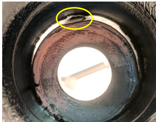
Figure 1: Anomaly found inside surface at the mold injection port one of the unfaulted 750kcmil T-bodies (left picture, yellow circle). The anomaly appeared to be a U-shape crack completely penetrating the semiconducting material (Faraday cage). Note the damage/crack continued into the insulation material but had not failed yet.
