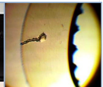
Electrical tree (carbon path) 50% through cable insulation
